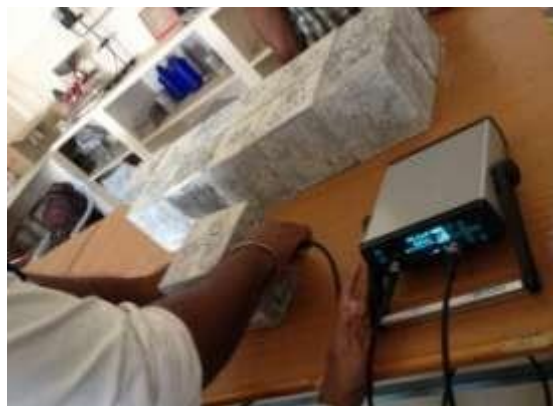
“Fig.3.2 Ultrasonic Pulse Velocity test of cubes
